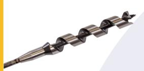
This high quality auger bit may become one of your most popular drill bits. Fabricated by Freeform using advanced manufacturing techniques, this bit includes an integral lead screw with course threads for precise drilling. The lead screw minimizes bit drift or "walk" and will help "pull" the bit through wood, taking less effort by the installer. The bit is made of a
