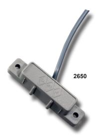
Using no mechanical parts, the GRI Sensors are triggered by a moisture bridge across the sensor contacts. The GRI Sensor can be installed to detect a layer of liquid as minute as 1/16 of an inch in depth.
