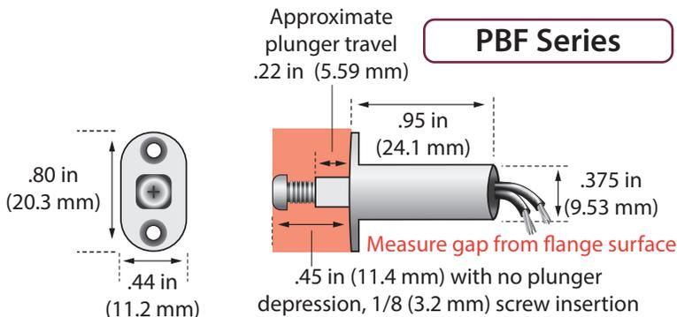
**CAUTION** For best performance, slightly over drill the hole for the switch and carefully clear hole of all debris. Too snug of fit can cause interference with switch operation. Do not paint the switch. Do not apply lubricant to the switch as this could hamper or restrict performance. These switches are not recommended for bottom track of windows or sliding doors.
