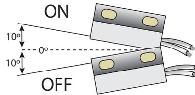
The GRI RoHS Tilt Switch fits a variety of applications where accurate detection of tampering is critical. The GRI 4561R was designed for use in a closed or open loop zone. The switch is incredibly durable and is hermetically sealed. Operation is based on the tilting of the sensor more than 10°. Using the wires as a reference point, tilt the switch toward the wires and the circuit is closed. Tilting away from the wires opens the circuit.
