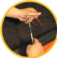
Tying wire to the flexible wire loop allows you to guide or pull the wire through tight and difficult paths, such as dashboards, framing, under seats, trunk spaces for stereo installation, trailer hookups and more.
